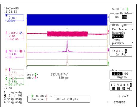
Figure 1– The mean squared (Area) and rms( sdev) jitter of a 10 MHz carrier modulated by a 100 KHz sine burst with a duty cycle of 50%.
